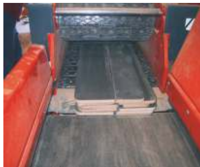
Chain link infeed for timber waste and chipboard stacks
