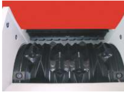
V-rotor, Ø 368 mm
