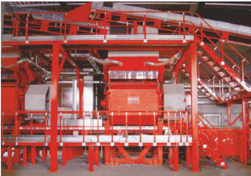
Core of the plant: the FineCut secondary shredder.
